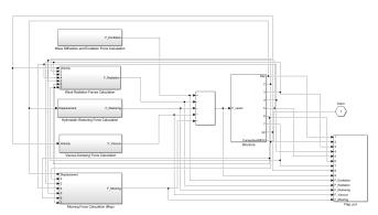
**(b)** An altered version of the model of Figure 1a, where we artificially resolved all buses and sub-buses up to the elementary signal lines. On the one hand, there are fewer blocks as the bus creators and selectors are removed. On the other hand, various new signal lines, block inputs, and outputs are now part of the diagram. Many of the signal lines cross other lines, and it is hard to discern which blocks are connected by which lines.
